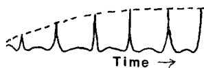
Fig. 9. Schematic illustration of gradual change of peak energy at the anvil site with time during a period of induced fitting.
